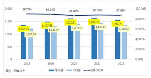
ii.2022 PTI recycled 87.61% waste water during dicing and grinding process.
